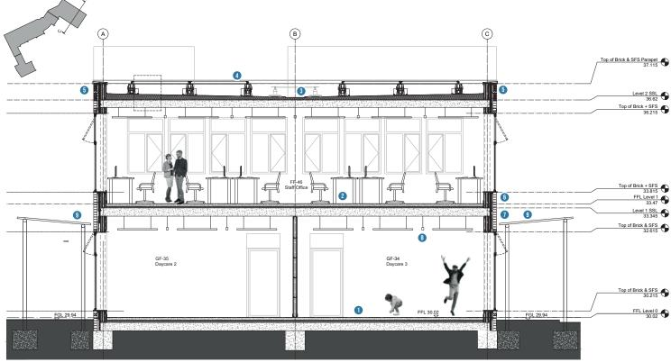
1 GROUND FLOOR Vinyl on 75mm Screed with UFH on 75mm Insulation on DPM on Concrete Slab
